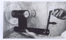
Figure 4.10 Lok-test equipment (photograph by courtesy of Lok-tew sindso
